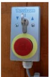
Control unit composed of key-switch with Emergency-off in dead-man's control and with cabling to the hydraulic power unit.
